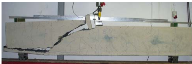
Crack pattern after failure of the experiment (left) and numerical results (right)
